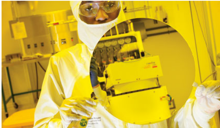
A bare, polished Si wafer
