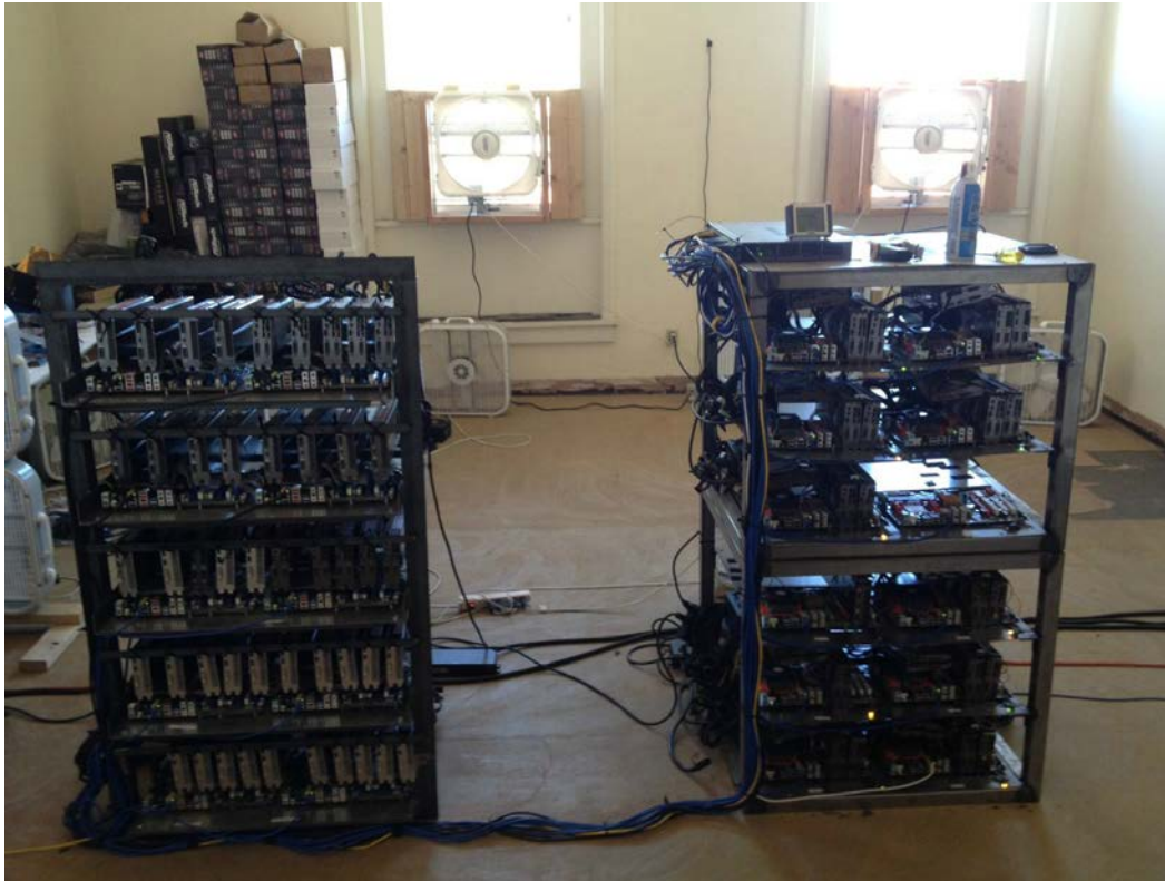
Figure 5.7: A home-built rack of GPUs used for Bitcoin mining. You can also see the fans that they used to build their cooling system. Source: LeonardH, cryptocurrenciestalk.com.
